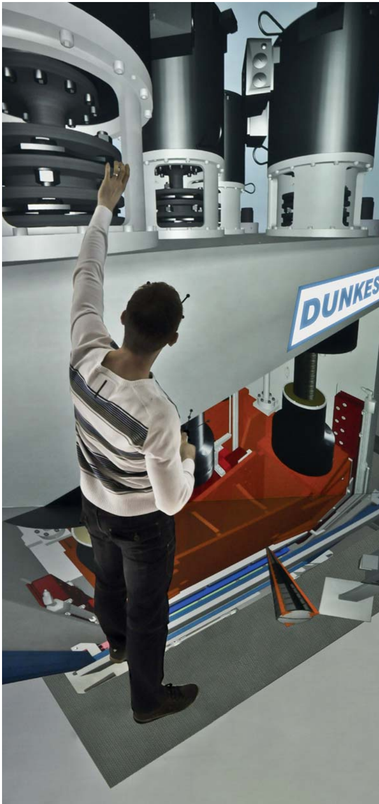
VR model of a spindle press to visualize manufacturing processes
