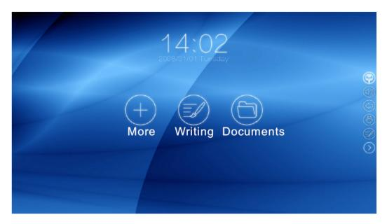
Upon startup, the machine will enter the main Android interface by default, as shown in the figure above. Under other signal sources, you can return to the main Android interface by directly clicking the right-side menu. The system also supports switching to the main Android interface by using the remote control or the button board on the machine.
