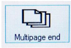
Please note, during scanning in the multipage mode, the single pictures will be stored temporary in the local folder c:/program\_data/.... With tapping on „**Multipage end**“ the files will be saved to the usb stick in one file.
