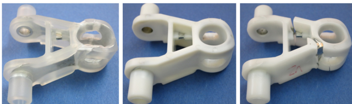
Figure 13: Hybrid chain links after quasi-static tensile testing: PP/Zinc (left), PBT/Zinc (center), POM/Zinc (right)
