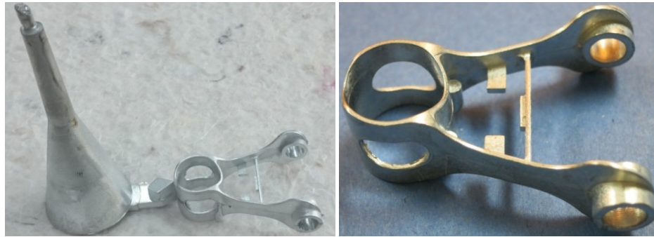
Figure 9: Cast blank with gate system (left), reinforcing structure ready for injection moulding (right)
