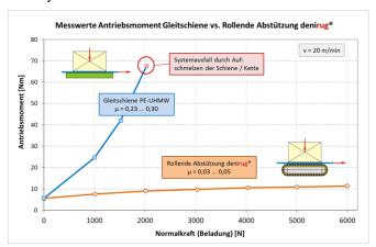
The straight RCT-elements of denirug® are vertical supports for chains and straps, especially in heavy load applications. Due to the extremely low resistance, the operating power can be significantly reduced up to 80%. At the same time, the range of application is increased and as a result of the diminished drag force clearly lighter and lower priced mat chains can be used.
