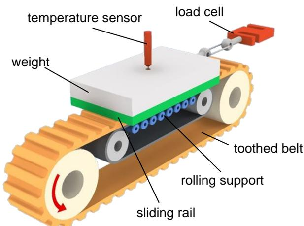
The experimental layout described makes it possible to record the friction force directly by using a load cell. The determined measured values are transferred to a computer which calculates the coefficient of friction using the quotient of friction force and weight force. Additionally the temperature of the wear couple is logged by a temperature sensor which is placed directly in the sliding rail. To prevent a further heat input the toothed belt runs on a rolling support.
