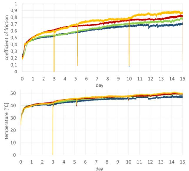
Besides the long-term recording of the progression of cof and temperature also the wear of the fabric coating and the sliding rail is evaluated. For this purpose incident light microscopes are available at the professorship of Materials Handling & Conveying Engineering. Furthermore there are laser microscopes which make it possible to do three-dimensional images of the surface topology of the fabric coating.
