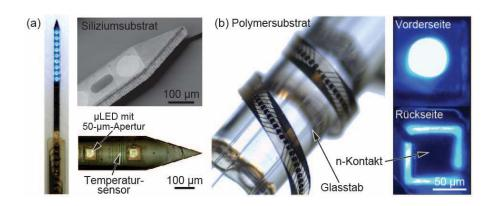
µLED-Arrays on (a) siliconbased and (b) flexible epoxide-based substrates comprising up to 144 µLEDs per optical probe.
