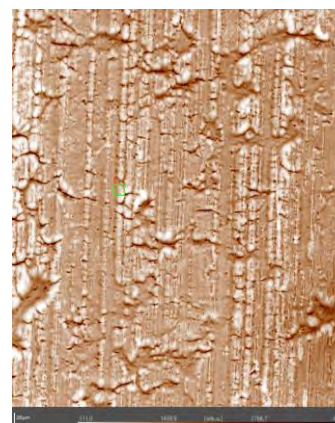
Fig. 1. Ellipsometric contrast micrograph of an oil film on a technical metal surface.
