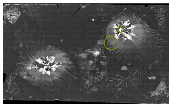
Fig. 1. Ellipsometric contrast micrograph of the complete sample with thin thiophene crystals on silicon with SiO 2 (d = 300 nm).
