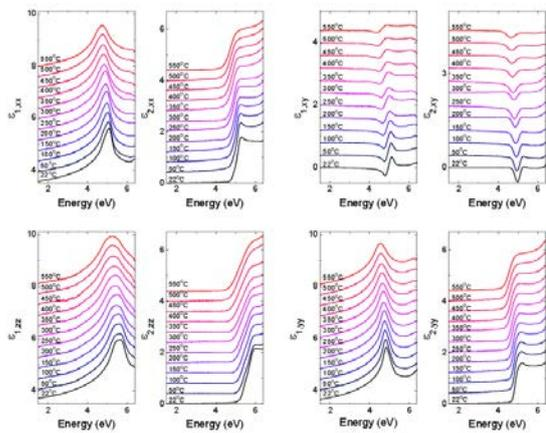
Figure 1: Real and imaginary components of the dielectric tensor elements,  $\epsilon_{xx}$ ,  $\epsilon_{yy}$ ,  $\epsilon_{xy}$ , and  $\epsilon_{zz}$  for room temperature (black) to 550°C (red) determined by generalized ellipsometry. The functions were shifted vertically by increments of 0.4 with respect to each other for convenience. Ref. [2]
