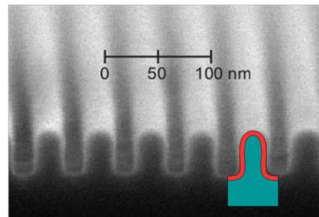
Fig. 1. Comparison of a silicon grating profile (green: silicon, red: silicon oxide) reconstructed from scatterometric measurement data with a cross-section SEM image obtained at an identically processed sample.
