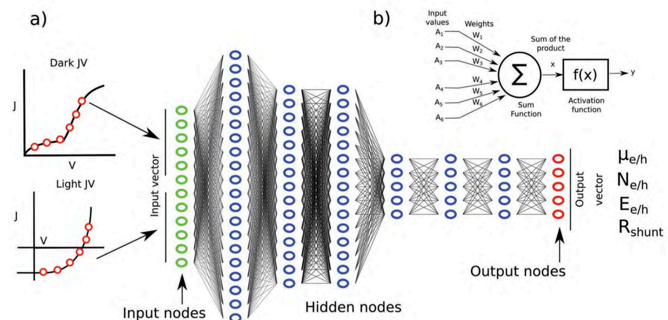
Scheme of the neural network, which is trained with simulated data and serves to determine the physical solar cell parameters.
