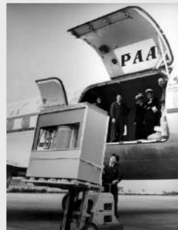
1956 – IBM 350 Magnetic storage (5 MB)
