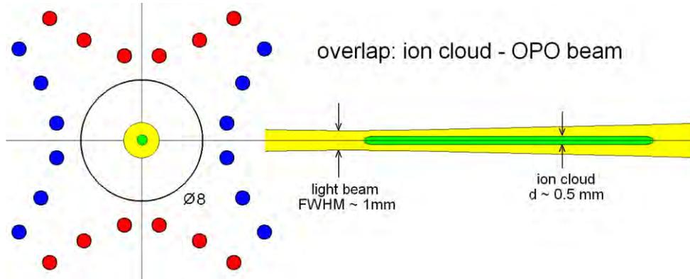
**Figure S1.** Overlap between the photon beam (yellow) and the ion cloud (green). The inhomogeneous rf field of the w4PT confines the ion cloud very close to the center line of the linear quadrupole. The broader laser beam surrounds the ions. The influence of space charge and a non-ideal beam profile of the OPO output are discussed in the text.
