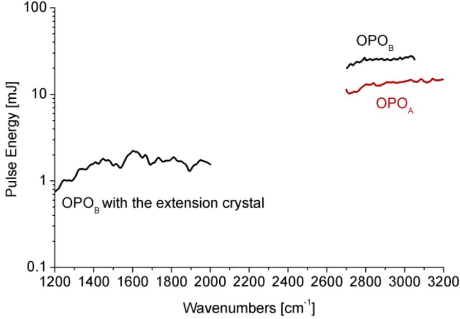
**Figure S2.** Energy per light pulse determined after the exit window of the instrument and corrected for the calibrated transmission trap - exit window.
