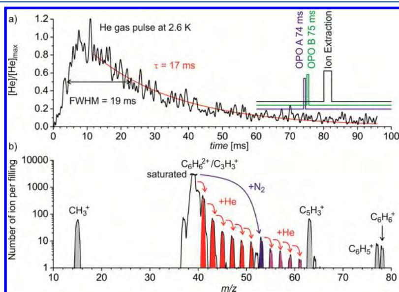
**Figure 1.** (a) Time sequence. The experiment is operated at the repetition rate of two synchronized Nd:YAG lasers (10 Hz). Together with a pulse of He gas, ions are injected into the trap.  $[C_6H_6He_x]^{2+}$  complexes are mainly formed in the first 30 ms. At 74 and 75 ms the two IR light pulses (10 ns) interact with the ions, which are extracted at 80 ms. (b) Mass spectrum of the ions after 80 ms trapping time (without irradiation).
