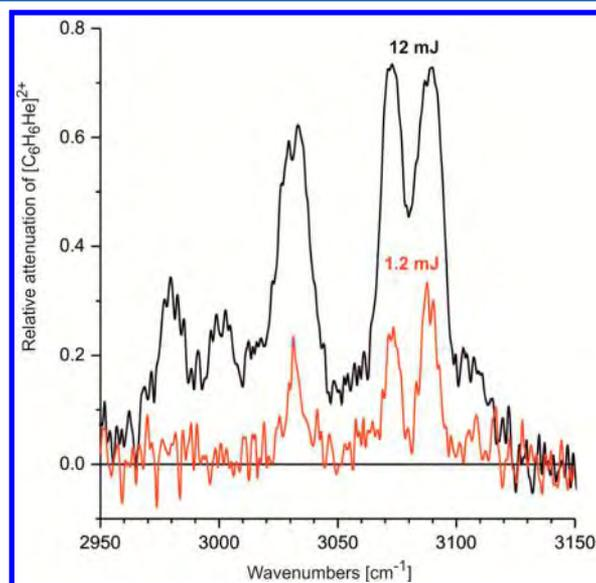
**Figure 2.** Relative number of fragmented complexes at the two indicated pulse energies of the IR light. With the 10 times more intense pulse, the lines are significantly saturated and power broadened. The two lines at the left do not show up with 1.2 mJ and are assigned as combination bands.
