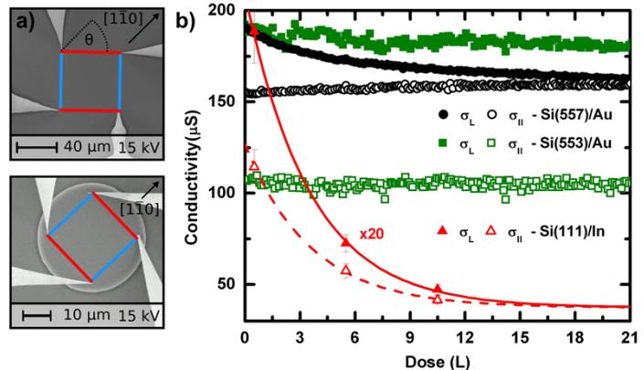
Figure 1: a) STM tips placed in square configuration on an unconfined In/Si(111) surface (above) and confined circular In/Si(111)-mesa structure (below). b)  $\sigma_{||}$  and  $\sigma_{\perp}$  versus O<sub>2</sub> dose for the Si(111)-4x1-In system, 0.48ML Au phase on Si(553) and 0.2ML Au phase on Si(557).
