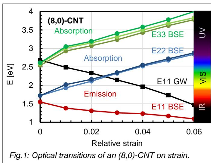
Fig. 1: Optical transitions of an (8,0)-CNT on strain.
