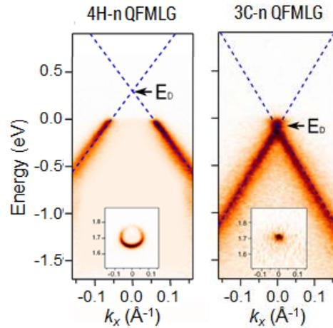
Fig. 1:  $\pi$ -bands of graphene on hydrogen-terminated, n-type 4H-SiC(0001) and 3C-SiC(111) probed by ARPES in the vicinity of the K-point of the hexagonal Brillouin zone. The position of the Dirac point  $E_D$  is marked.
