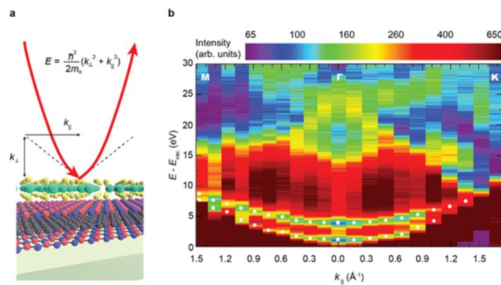
Fig. 1. **a**, Changing the angle of incidence of low-energy electrons onto a surface while recording their energy and reflected intensity yields insights into the materials unoccupied band structure. **b**, This ARRES measurement reveals, e.g., the bands of bilayer graphene and shows clear band quantization at low energies.
