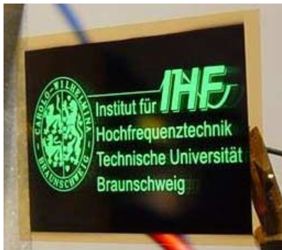
Figure 10: First large area OVPD-OLED displaying the Logo of TU Braunschweig processed on a substrate size of 35 x 50 mm 2 .
