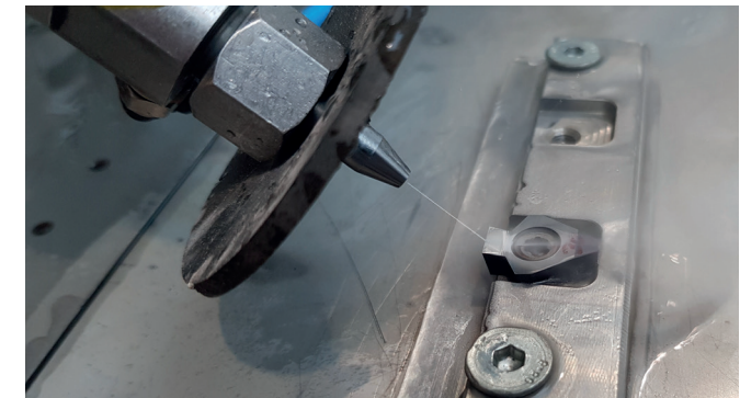
Cutting edge preparation with high pressure water jet
