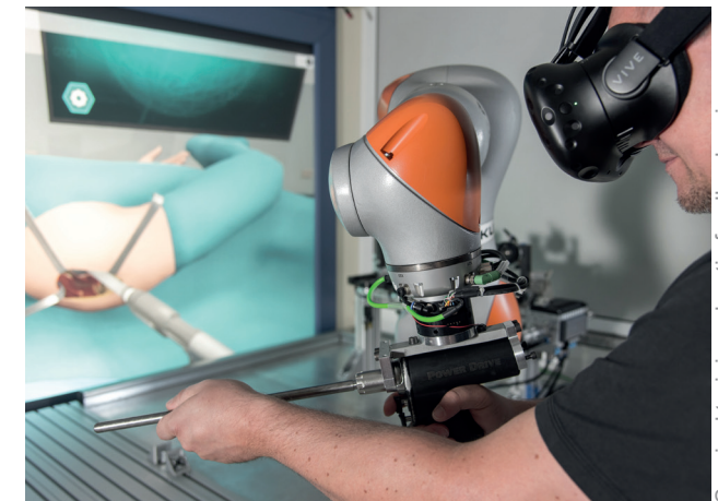
Surgical training - haptic feedback using a robotic arm
