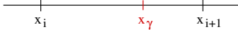
Figure 1: Graded refinement of an edge, with x_\gamma = (1 - \gamma)x_i + \gamma x_{i+1} , \gamma \in (0, 1) .
