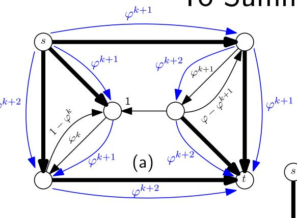
This flow has value  $2\varphi^{k+1} + 2\varphi^{k+2} = 2\varphi^k$
