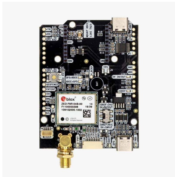
Figure 8: simpleRTK2B ZED-F9R GNSS receiver board (source: ArduSimple) [29].
