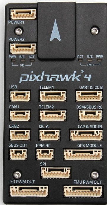
Figure 11: Pixhawk-4 flight controller used for UAV navigation and control [32].
