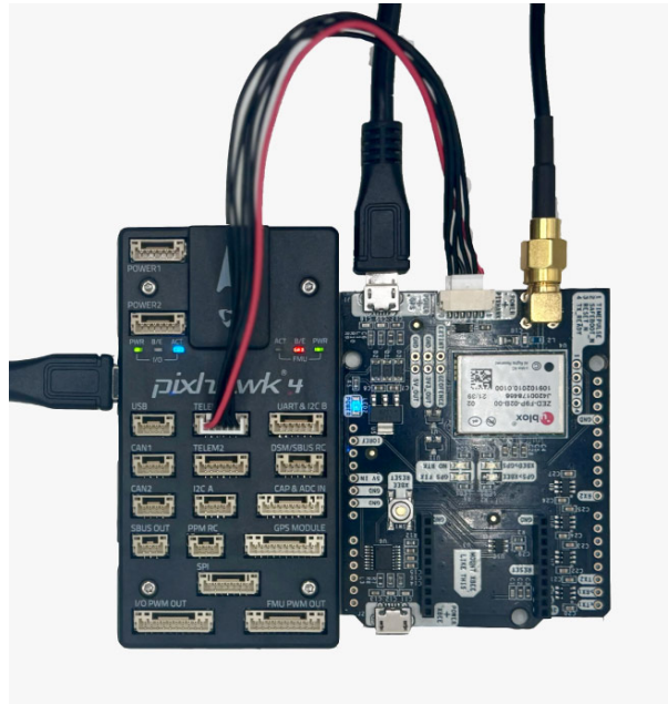
Figure 18: simpleRTK2B and Pixhawk configuration [37].
