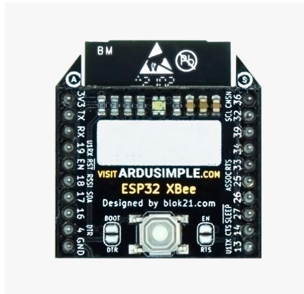
Figure 10: ArduSimple WiFi NTRIP Master used for RTK correction transmission [31].
