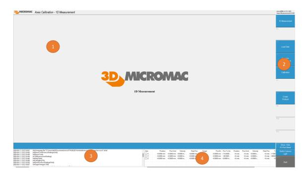
Figure 5.2.: Overview of the MMI implementation showing configuration/display panel (1), action buttons (2), log console (3), and axis status display (4)
