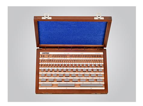
Figure 3.1.: Metric gauge block set
