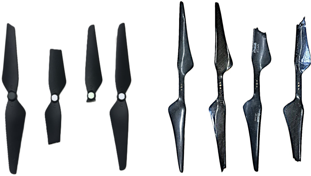
(a) Holybro X500's, from left to right: D3, D2, (b) Y6 AREIOM's, from left to right: H, D3, D1, H.
