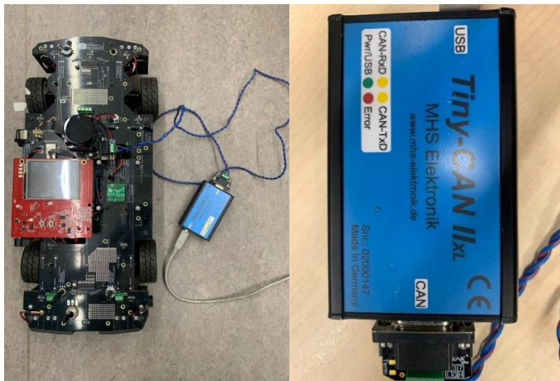
Figure 5.10: TUCminiCar with the Tiny Can hardware connected.
