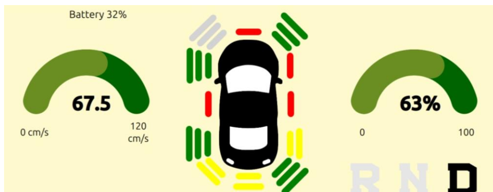
Figure 5.5: Lidar data displayed when speed >60.
