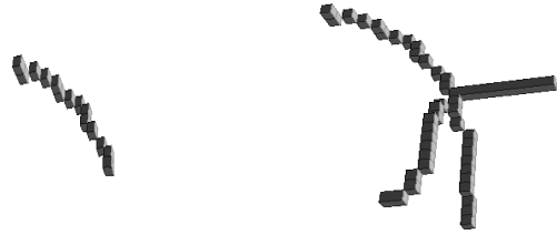
Figure 9: At left a single curve consisting of voxels is displayed, at right on the other hand several joined curves, which form a curve skeleton.
