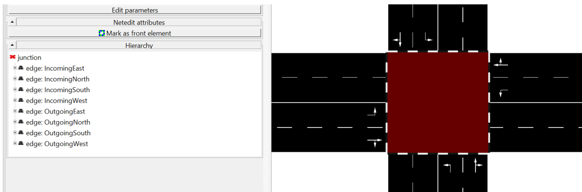
Figure 8.1.: netedit view of network file and edge definitions for layout from Fig. 3.1.
