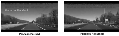
Fig. 5: Lane Curvature Detection in Critical Road Condition: Radius to left and right lane curvature is 330m and 493m; curve to the right (left), Radius to left and right lane curvature is 818m and 943m (right)
