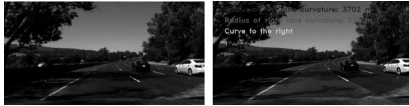
Fig. 4: Lane Curvature Detection in Low Light Condition → Radius to left and right lane curvature is 3702m and 3796m; curve to the right
