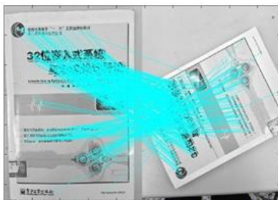
Fig. 4. Feature matching under rotation condition
