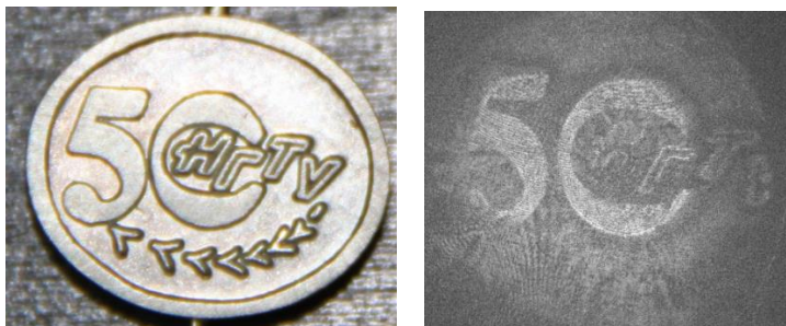
Figure 4. Left source object, right: the result of restoring the actual image from the mathematical hologram.
