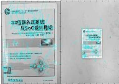
Fig. 2. Feature detection of the same objects under different scale
