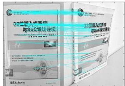
Fig. 5. Feature matching under perspective transformation
