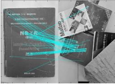
Fig. 8. Feature matching under the condition of rotation, cover, translation and scale changes
