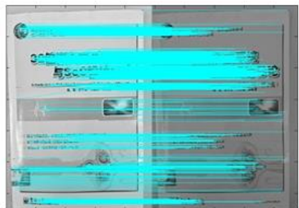
Fig. 7. Feature matching under the condition change of brightness
