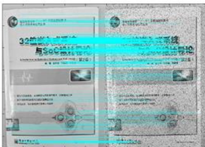
Fig. 6. Feature matching under the conditions of noise
