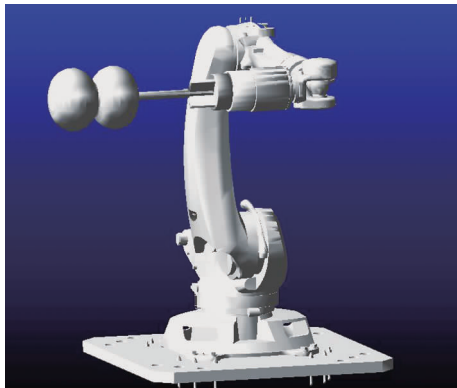
Fig. 7 The robot winding position while the starting angle of six joints are respectively 0^\circ , -90^\circ , 90^\circ , -90^\circ , -90^\circ , 0^\circ
