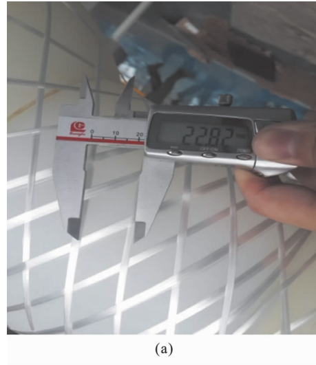
Fig. 10 Winding pattern of geodesic for a cycle of dumbbell core mandrel using a single yarn while length of free fiber is 150 mm, winding pattern is -5/3 and width of yarn is 50 mm
