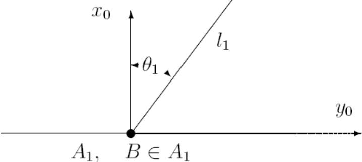
$$M = \begin{pmatrix} c_{12} & -s_{12} & 0 & l_2 c_{12} + l_1 c_1 \\ s_{12} & c_{12} & 0 & l_2 s_{12} + l_1 s_1 \\ 0 & 0 & 1 & 0 \\ 0 & 0 & 0 & 1 \end{pmatrix}$$
