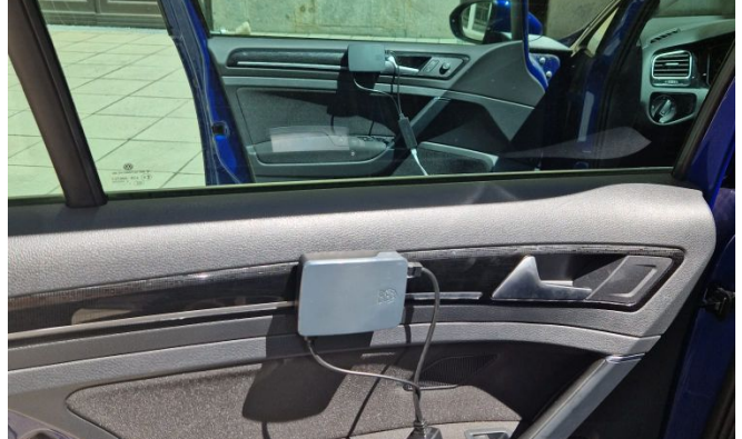
Fig. 5: CSI sensors 1 and 6 temporarily mounted on the driver's side doors by hook-and-loop fasteners.
