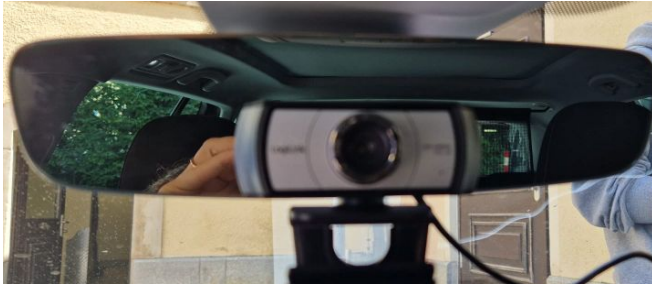
Fig. 7: Camera mounted on the rearview mirror pointing at vehicle’s interior.
