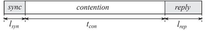
Figure 4: Every transmission cycle consists of three parts: sync, contention phase and reply. A sync message informs vehicles about the length of the contention phase, where these can transmit a request message to the RSU. At the end of the cycle, the RSU replies to all vehicles with a single reply message.
