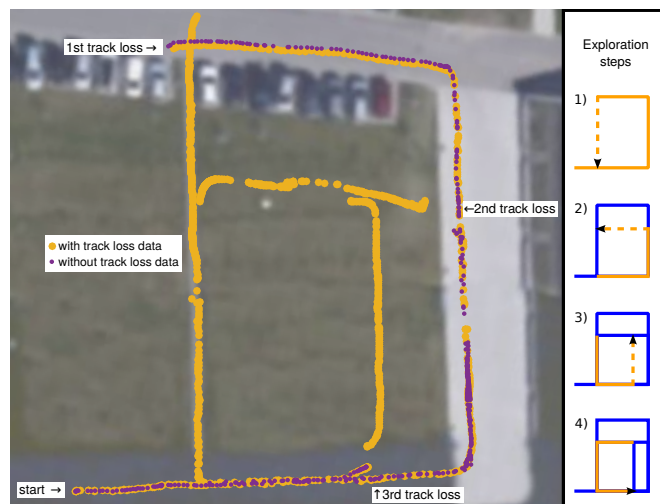
Fig. 1. Comparison of the original ORB-SLAM (purple) with a modified version (yellow) for a proof-of-concept experiment – each point represents the position of a keyframe on the track. Each track loss is caused by a fast rotational movement. The used extension of ORB-SLAM, Reverse Replay , is presented in section III. The right column gives an intuition about the traversed path; dashed lines mark path segments during track loss.
