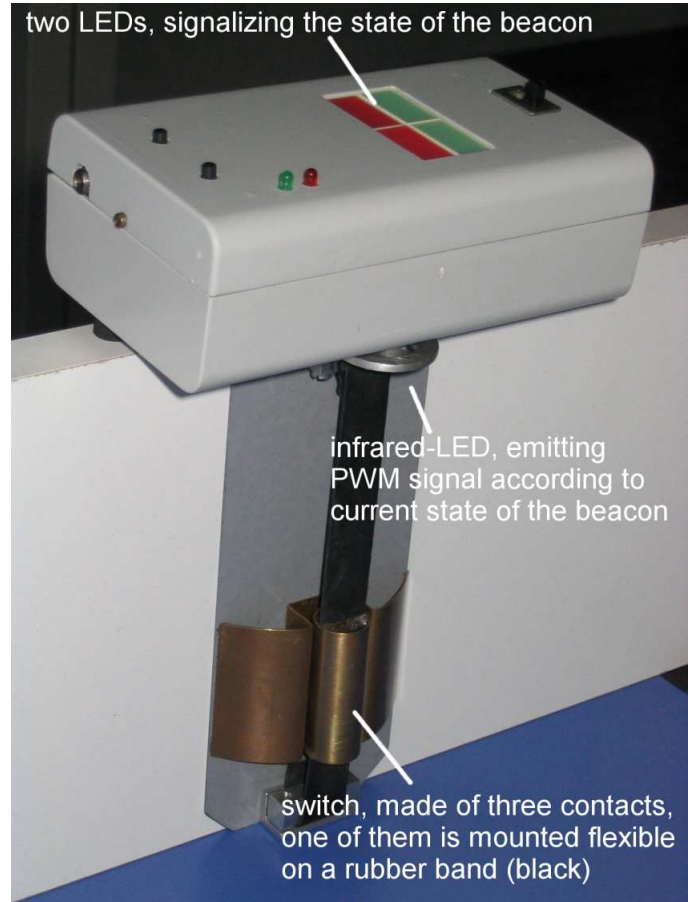
Fig. 4. A beacon. Notice the big red and green LED on top of it. They show the actual state the beacon is in. The infrared-LED is just beneath the white body. The switch is at the bottom, so that the robots can simply drive against it.
