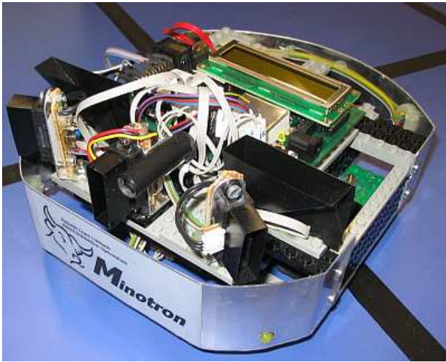
Fig. 7. A close-up of the winning robot, Minotron. It was based on LEGO bricks, but used a lot of non-LEGO sensors like GP2D120. The runner-up was made from LEGO bricks as well.
