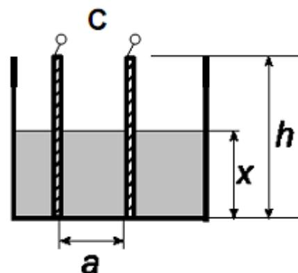
Because the dielectric permittivity  $\epsilon_r$  of the liquid and the distance  $a$  of the plates are not precisely known, a calibration is required. Calibration should be done with low effort.
