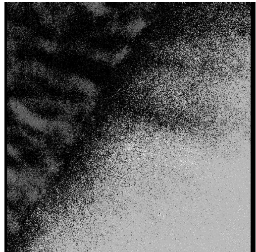
Figure 4: EELS mapping of sample C, same area as in fig. 3; black = O, grey = Pt, light grey = Si.
