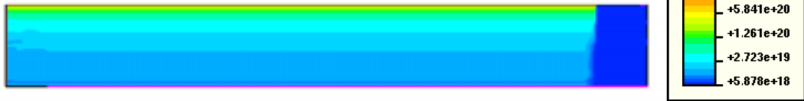
Fig. 4a: optical generation rate within simulation model of conventional solar cell
