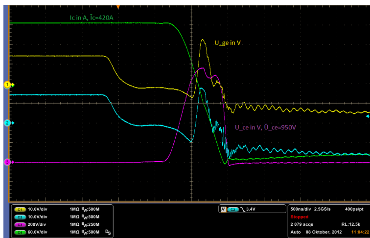
Figure 1: Gate voltage and collector-emitter voltage during switching-off, collector current 420A. PrimePACK2-module rated voltage 1200V, adjusted voltage peak \hat{U}_{ce}=950V
