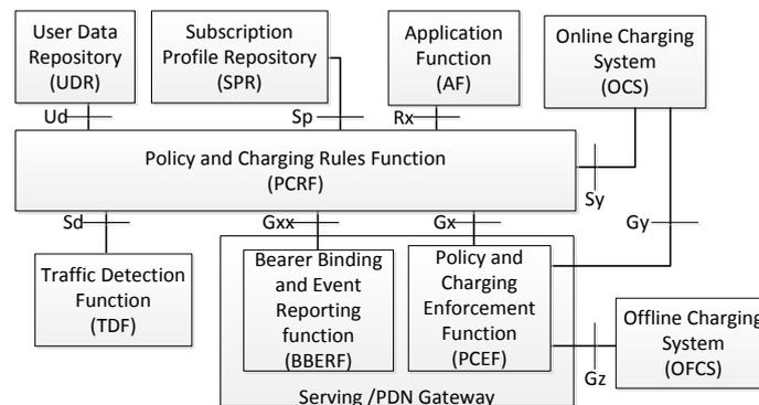
**Fig. 1.** 3GPP PCC logical architecture after [2] and [4]
