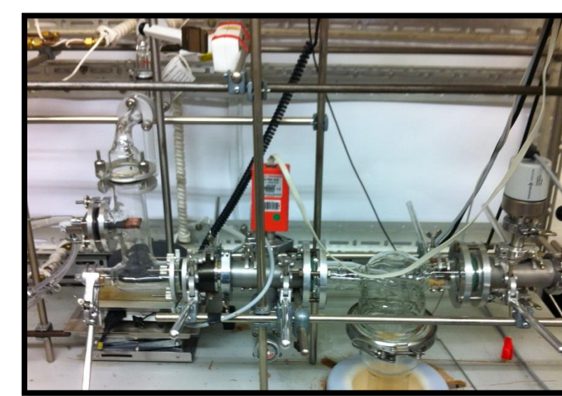
Fig. 7: Home-built vertical cold-wall CVD-reactor.
