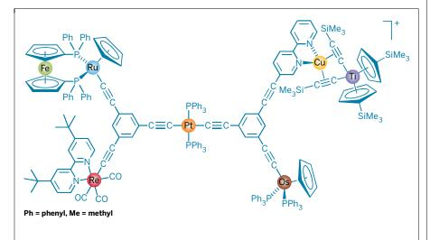
**SEVEN IN ONE BLOW** This novelty complex has a record seven different metals on board; it was made via a string of various chemical transformations.
