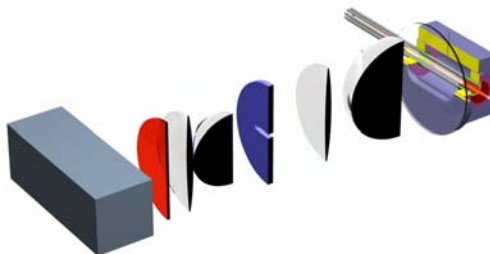
Fig. 3: The optical detection system uses a photomultiplier (R1527P) for single photon detection. The quantum efficiency is 10 %, the visible trapping volume is also about 10% of total storage volume, and the collection efficiency for photons is 2% (through the octopole rods).
