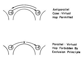
Fig. 2. Virtual hopping as the origin of superexchange.
