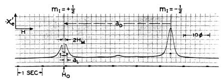
DEMONSTRATION OF THE INHOMOGENEOUS BROADENING IN P-DOPED SILICON ( $\rho=0.25\,\Omega$  Cm, T = 1.2° K, H<sub>0</sub> = 3000 Ø) IN THE ENDOR TECHNIQUE SPIN PACKETS ARE FLIPPED AS INDICATED BY ARROWS
