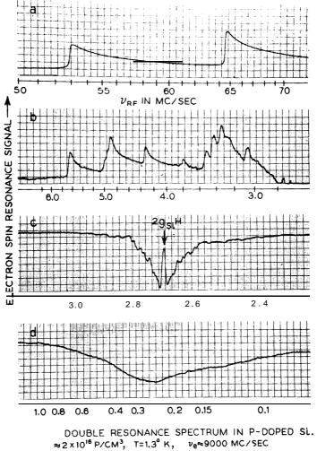
≈2×10<sup>16</sup> P/CM<sup>3</sup>, T=1.3° K, ν<sub>e</sub>≈9000 MC/SEC Fig. 11. a) "Hole-digging" and ENDOR spectrum. While saturating a specific frequency
