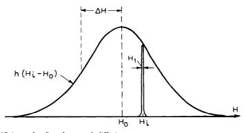
Fig. 13. "Spin packets" and spectral diffusion.
