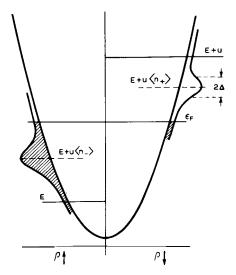
Fig. 5. Spin-split energy levels in the magnetic case.
