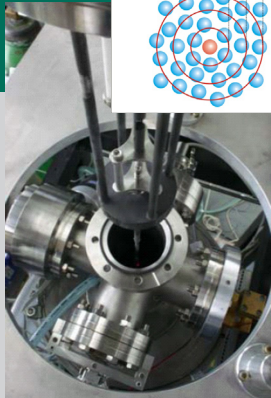
Sample transfer window of a high temperature viscometer
