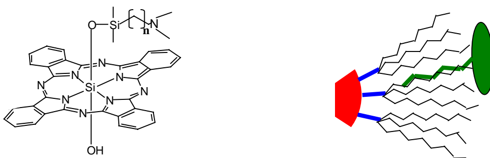
Figure S2. On the right is the backbone structure of the Silicon Pc used in this study, where the total linker chain length is described as the distance between the Pc ring and the amino group given as # bonds = n + 3 (i.e. n methylene groups together with an oxygen, a silicon and nitrogen atom). On the right is the schematic diagram of the interdigitization process of the capping layer (e.g. TOPO) with the linker chain of the Pc.
