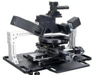
Fig.2 M-2000 Ellipsometer, which will be used to determine the ellipsometric data [2]
