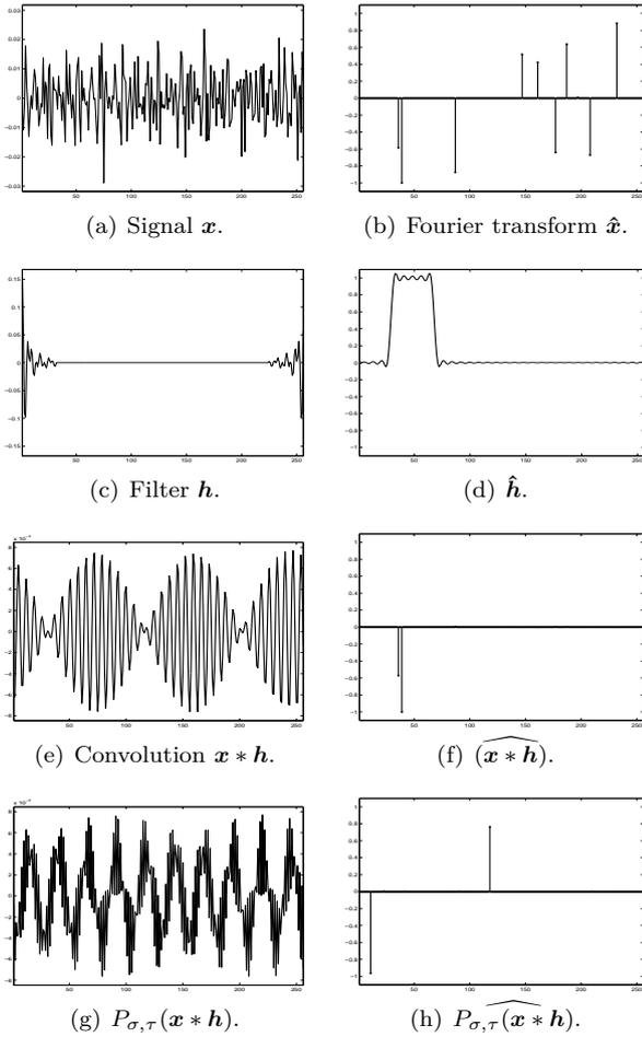
Figure IV.1. **Example step of the split Prony-like method.** In step  $b = 2$  of  $B = 8$  computation steps, the signal  $\mathbf{x}$  of length  $N = 2^8 = 256$  (a) with  $K = 10$  non-zeros in its Fourier transform  $\hat{\mathbf{x}}$  (b) is convolved with the filter  $\mathbf{h}$  (c). The resulting vector  $\mathbf{x} * \mathbf{h}$  (e) is randomly permuted. In all the subfigures only the real parts of the complex vectors are plotted.
