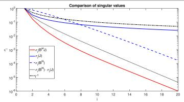
Semi-logarithmic plot of singular values of  $n \times n$ -matrices with  $n = 10^4$  supporting points representing **discretization matrices** of the operators *A*,  $B^{(H)} := H$  and *J*. **Singular values of A** = **H**  $\circ$  **J decay exponentially** in the numerical experiments.
